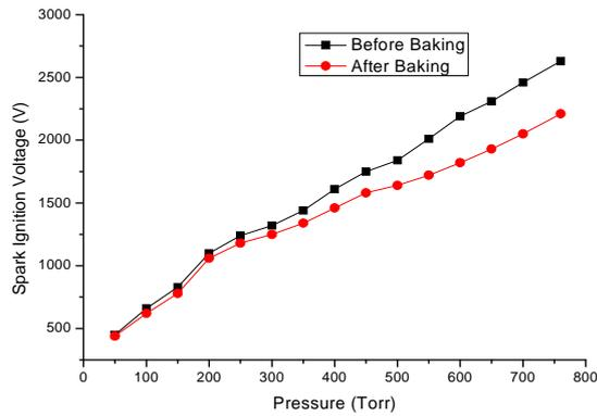
Fig.5. Spark ignition voltage versus pressure
