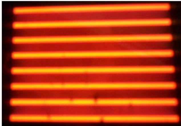
Figure 4. The coplanar barrier discharge process in neon.
