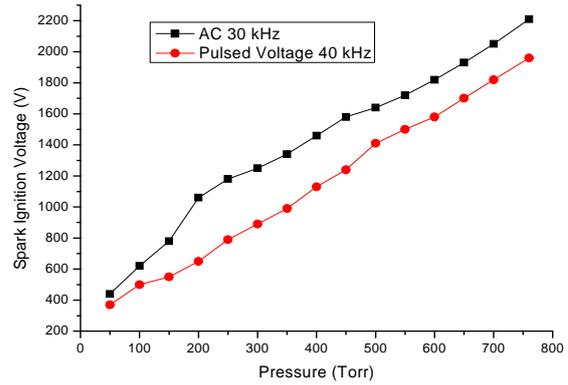
Fig. 6. Spark ignition voltage versus pressure
