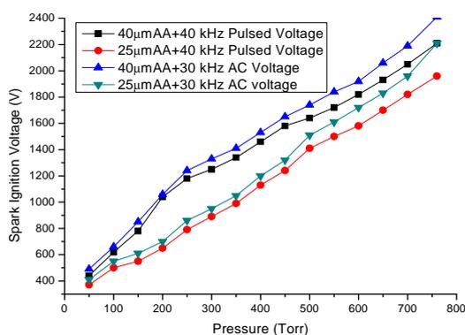
Fig.7. Spark ignition voltage versus pressure at different alumina thicknesses
