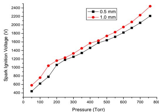
Fig. 8. Spark ignition voltage versus pressure at different electrode gap distances
