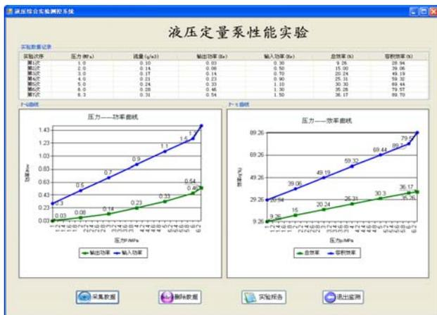
Figure 5 hydraulic fixed displacement pump characteristic experiment static curve
