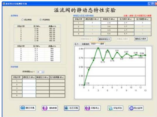
Figure 6 relief valve dynamic property curve diagram
