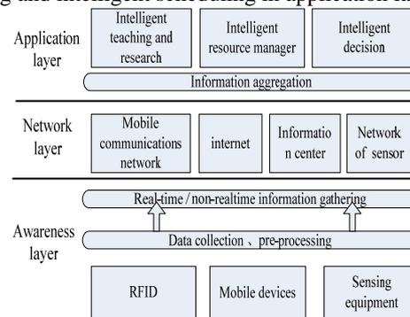
Figure 1. the system framework under the environment of IOT
