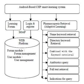
Fig.2. System functional modules
