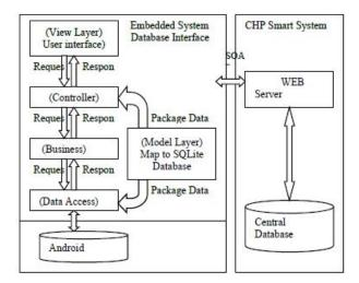
Fig. 1 System Architecture
