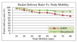
Fig. 6. Packet Delivery Ratio Vs. Node Mobility
