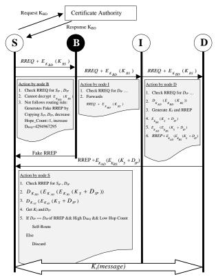
Fig. 5. Algorithm to secure routing protocol and data transmission
