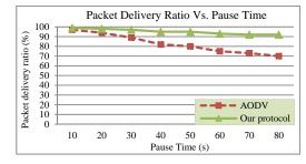
Fig. 7. Packet Delivery Ratio Vs. Pause Time
