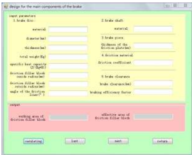
Figure 5. Major parts of the brake design
