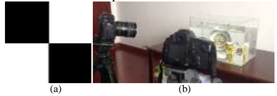
Figure 3. (a) Checkerboard marker used for interface normal calibration. (b) Experiment configuration
