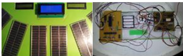
Figure 2. (a)The prototype system of green energy surveillance system (exterior) (b)The prototype system of green energy surveillance system (interior)
