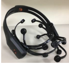
Figure 1 | EMOTIV EPOC (wireless portable EEG headset).
