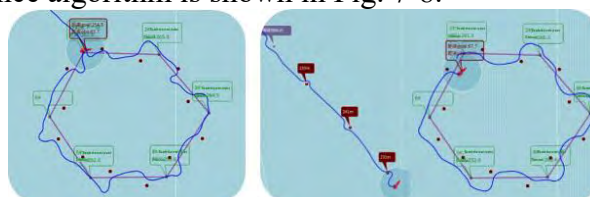
Fig. 7 Obstacles avoidance trace of USV when using traditional artificial potential field algorithm (left) and using the improved algorithm in Taihu Lake (right)
