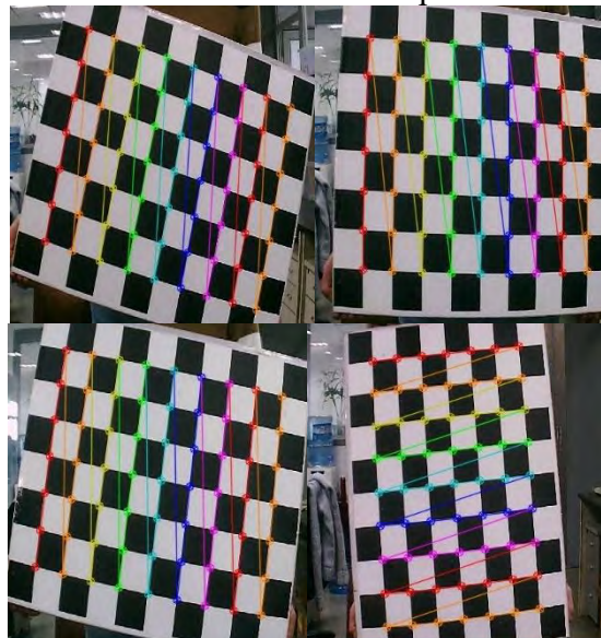
Fig. 6 Inner corner detection results of camera calibration image
