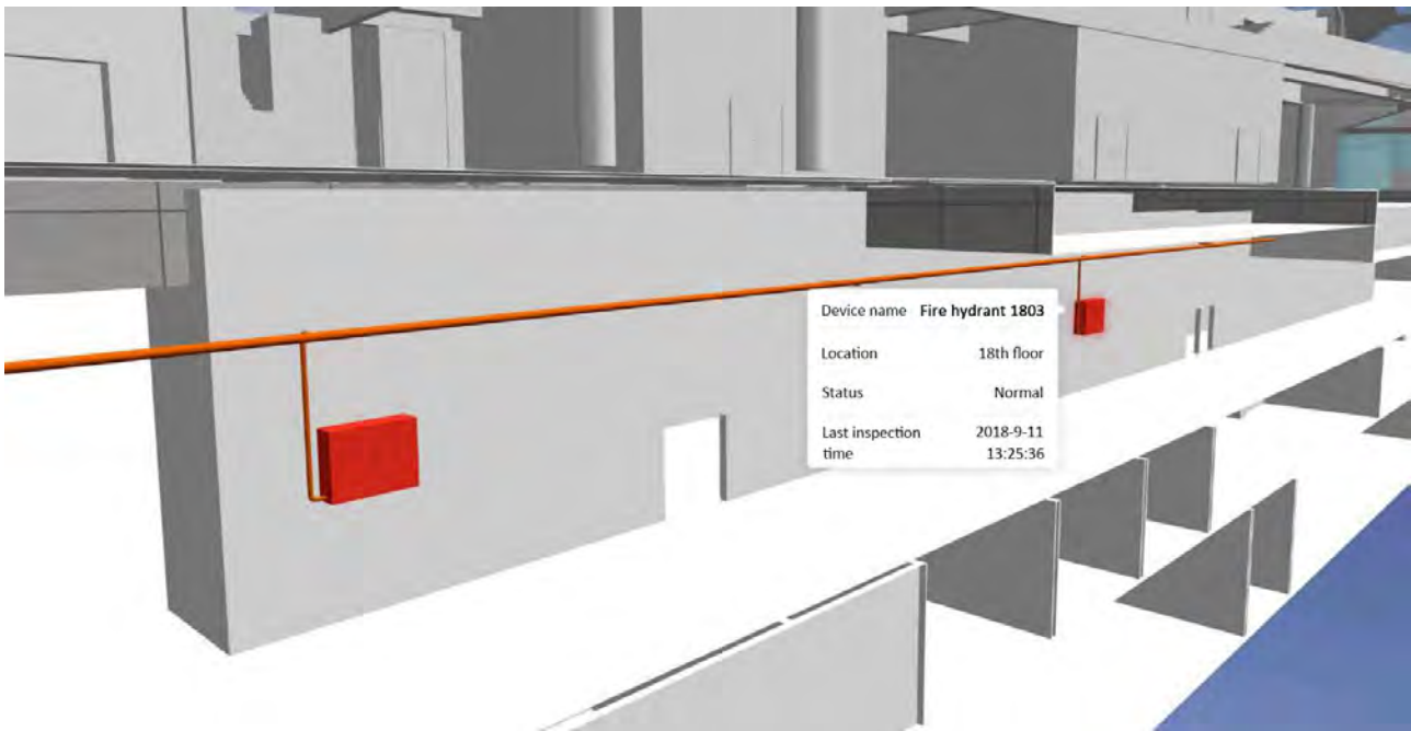
Fig. 2 IoT sensing data in BIM
