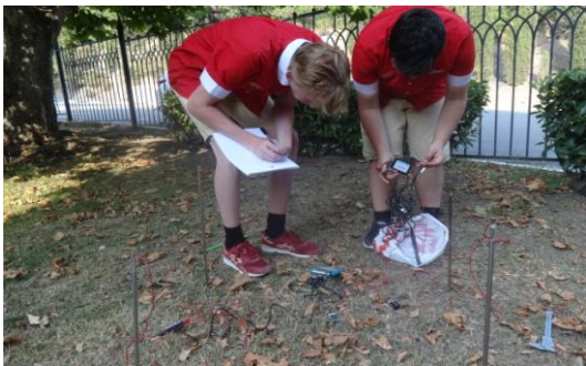
Fig. 5. Measurement of the conductivity of ground by Van der Pauw method
