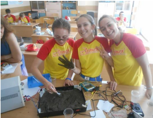
Fig. 4. Measurement of the conductivity of soil by Van der Pauw method
