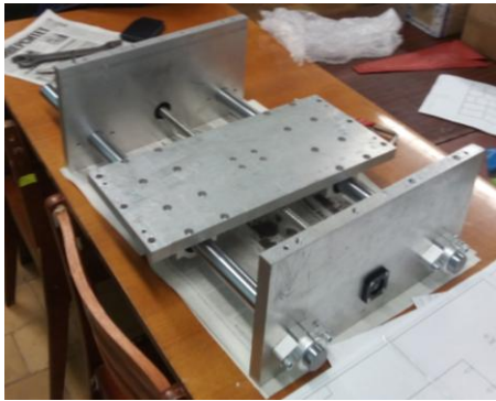
Fig. 3. The CNC-machine table development project result
