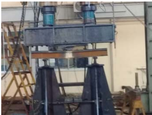
Fig. 8. Picture of specimen with joint type R260-R260 after static bending test
