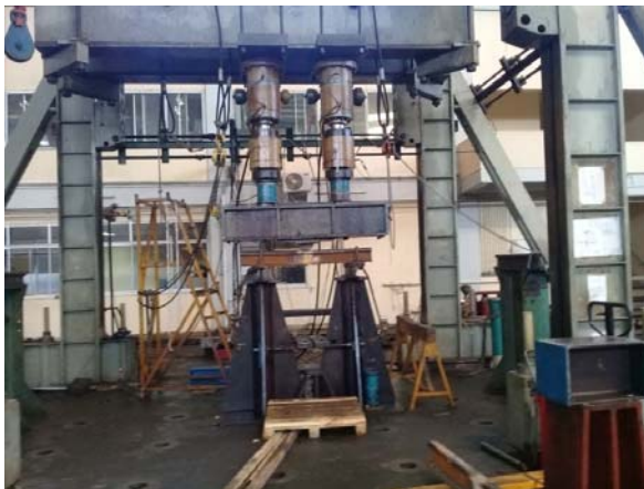
Fig. 3. Picture of test set up for static bending test
