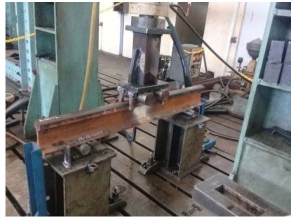
Fig. 6. Picture of test set up of fatigue test
