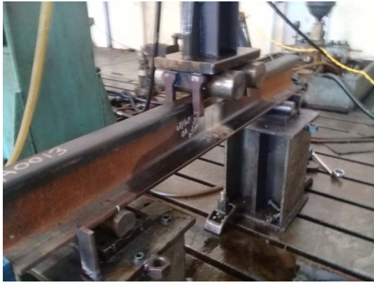
Fig. 7. Picture of specimen with joint type of R260-R260 after fatigue test
