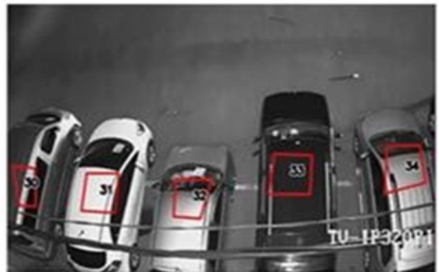
Fig. 6. Vehicle Parking Identification Results Using Smart Cameras At Night From the above test results as shown in Fig. 6, the test runs at night, the vehicle identification program runs quite well where the virtual red border shows the parking lot filled by the vehicle identified by the camera.
