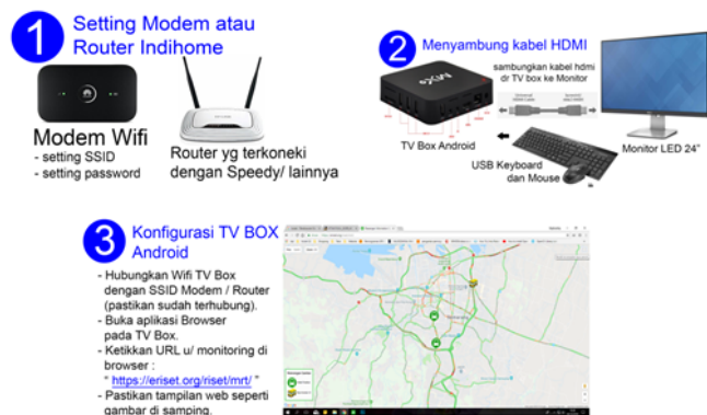
Fig.8. Configuration of monitoring system and passenger information system
