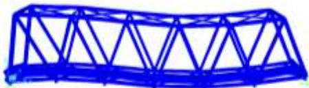
Fig. 6. mode shapes in X direction
