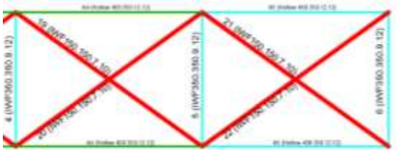
Fig. 23. Detailed of overstressed frame number 19-22 (IWF150.150.7.10)
