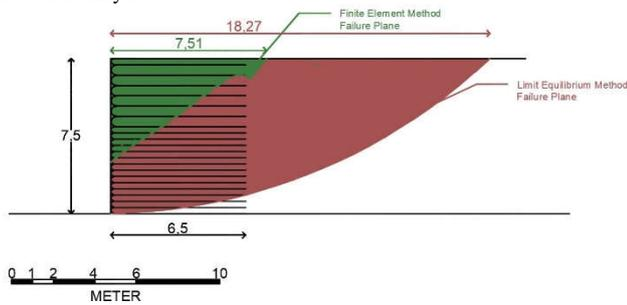
Fig. 12. Dynamic Failure Plane of MSWE Design Based on LEM and FEM
