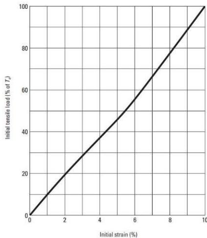
Fig. 9. Initial Tensile Load–Strain Master Curve for Polyester Geotextiles [14]
