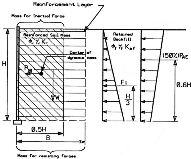
Fig. 7. Model Geometry and Force Distribution of MSWE with Additional Seismic Loading [11]
