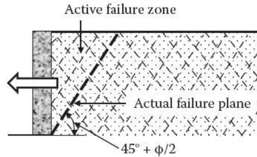
Fig. 2. Potential Failure Plane of an Active Conditioned Backfill [8]
