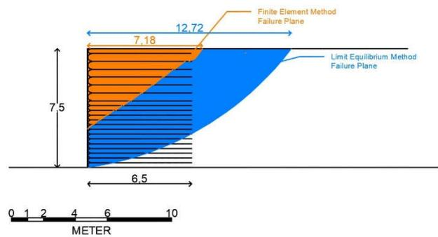
Fig. 10. Static Failure Plane of MSWE Design Based on LEM and FEM As a result, the PGA used for the analysis is reduced to 0.508. The analysis of dynamic stability is also separated into internal dynamic stability and external dynamic stability evaluations.
