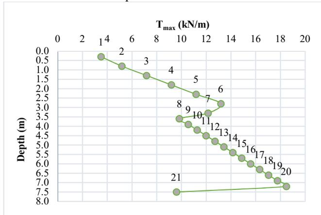
Fig. 11. Maximum Static Tensile Force ( $T_{max}$ ) Distribution Alongside the Geotextile Layer
