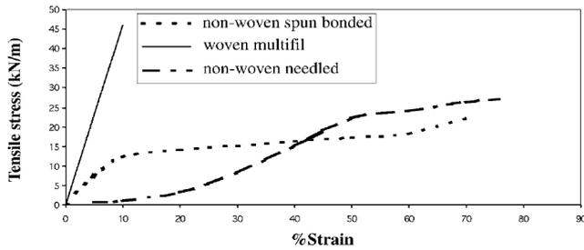
Fig. 1. Typical and Schematic Geotextile Strain-Stress Curves [5]
