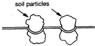
Fig. 3. Representation of Soil Reinforcement [10]
