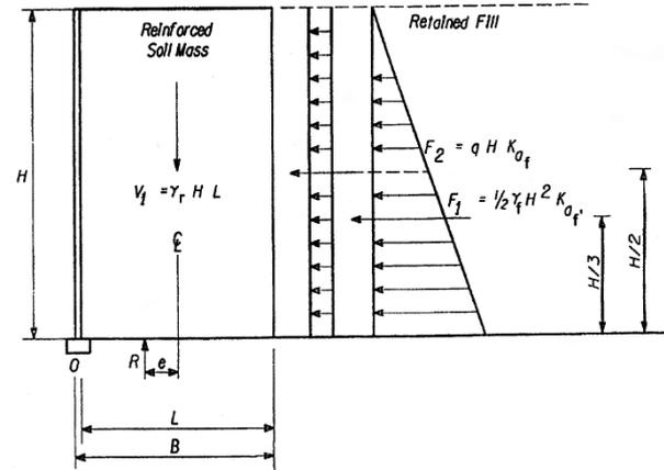
Fig. 6. Model Geometry and Force Distribution of MSWE Under Static Loading [11]
