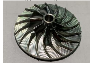
Figure 15. Micro integral impeller after machining
