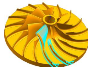
Figure 8. Blade finishing tool path of impeller
