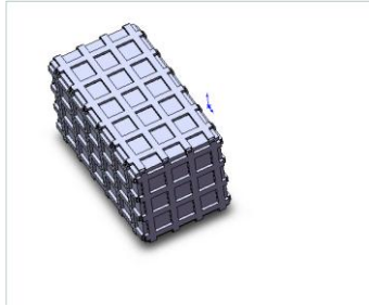
Figure 10. Drying chamber with a wall thickness of 15 mm and a rib spacing of 410 mm
