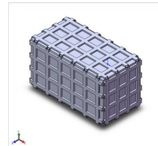
Figure 7. Drying chamber with a wall thickness of 8 mm and a rib spacing of 410 mm
