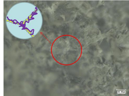
Figure 5. The depth digital optical microscopy of composite material (BN+MWCNT)/UHMWPE
