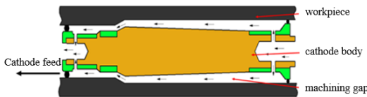
Figure 2. Physical model of variable cross-sectional hole electrochemical machining
