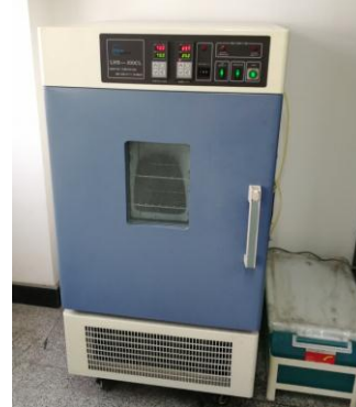
Figure 2. LHS-100CL constant temperature and humidity test chamber
