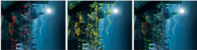
(e) Harris algorithm, SIFT algorithm, Harris-SIFT algorithm in this paper on the rotation of the image extraction effect
