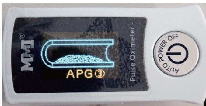
Figure 1 | Arterial stiffness index using the pulse oximeter SB200 device. The SB200 pulse oximeter also gives the ASI, which is again classified in six levels, with level 1 representing excellent condition and level 6 representing poor condition.
