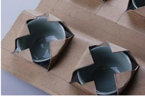
Fig. 10. Kungfu tea cup — part 1 of scroll packaging structure.
