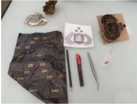
Fig. 13. Materials and tools used to make batik master stamp (carbon paper, HVS paper, 2B pencil, cutter, tweezers, hardboard cut, G glue, duplex/ Malaga paper. (Source: Studio of the Department of Textile at SMK Negeri 3 Kasihan, Bantul, Yogyakarta Photographer: Probosiwi, 2019)
