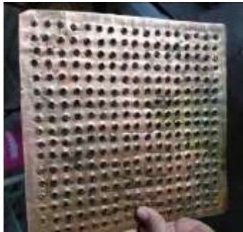
Fig. 7. A metal plate that functions as a filter for night dirt (wax) that has been heated in a pan or pan. The size of the slab is adjusted to the diameter of the pan or pan. (Source: Studio of the Department of Textile at SMK Negeri 3 Kasihan, Bantul, Yogyakarta Photographer: Probosiwi, 2019)
