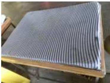
Fig. 8. A wetable that functions as a cloth base that is being stamped with a metal stamp. This table contains cold water that is stacked with a sponge and covered by a blanket cloth and covered by glass paper. The purpose of this table is made so that the process of tasting the fabric is not sticky because it is exposed to cold temperatures from glass paper. (Source: Studio of the Department of Textile at SMK Negeri 3 Kasihan, Bantul, Yogyakarta Photographer: Probosiwi, 2019)
