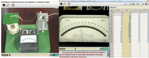
a) b) c) Figure 6 Windows of the laboratory work "Measurement of entropy during heating and melting of tin": a) installation; b) millivoltmeter; c) spreadsheet
