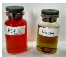
Figure 1. Qualitative anthocyanin test of rambutan fruit rind extract (HCl; left, and NaOH; right)
