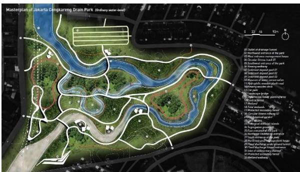
Figure 9 - A proposal designed to mimic a natural river system and leverage off its ability to deposit sedimentation (Fang Zihan)
