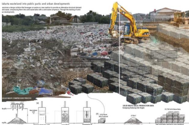
Figure 15 - Rather than trying to burn or otherwise remove the waste, the student here saw an opportunity to utilise waste as a building material (Chin Carissa)
