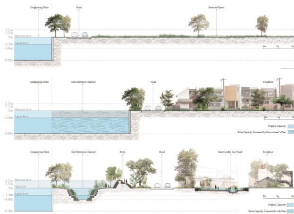
Figure 8 - Three sectional profiles on current (top), 2030 plan by Jakarta government (middle), and landscape-centric proposal (bottom) (Wang Haobo)
