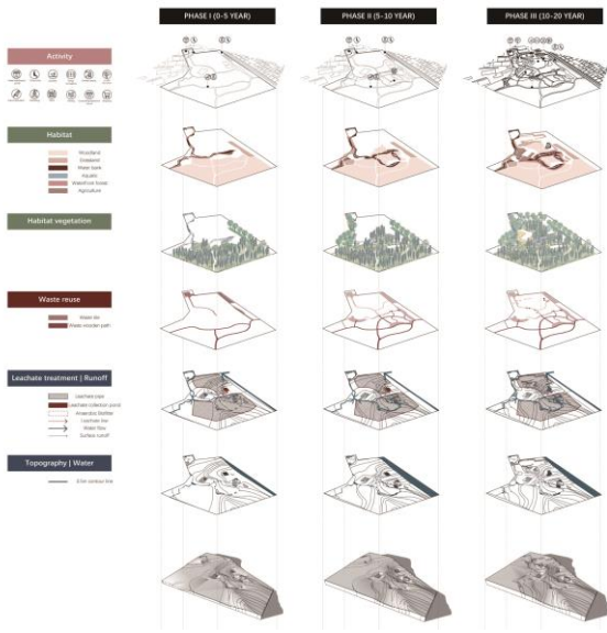
Figure 14 – A 20-year long phasing plan for the design layers introduced to rehabilitate the landfill site (Zhang Bingyi)
