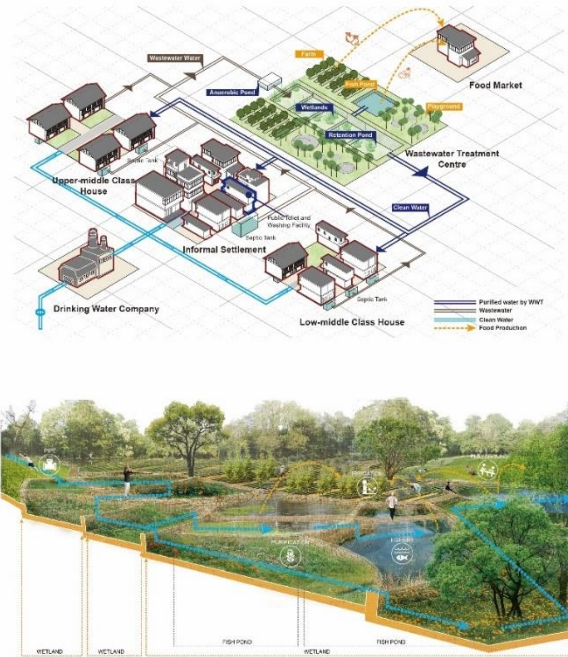
Figure 7 - Diagram of circular water flow between neighbourhoods and public park (top). Visualization of terraced wetland system in the park for water cleansing purpose (Lyu Jiawei)
