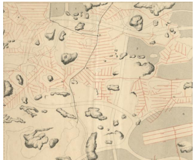
Figure 4. Map of Drainage System of Central Park, 1858. The red lines represent the tile drains, red circles are the silt basins, and the heavy black lines indicate the sewers.
