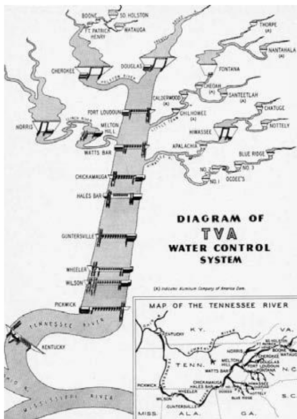
Figure 5. Diagram of the TVA water control system. 26 dams work as a unit.
