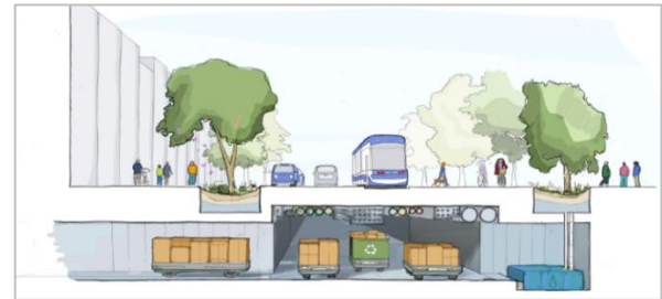
Figure 3 Concept of an underground delivery system Source: Toronto Sidewalk Schematic Pieces [30], downloaded February 23, 2020
