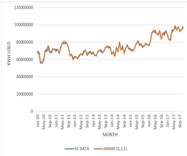
Figure 3 Plot of the monthly electricity consumption data of Cagayan de Oro City from January 2010 to December 2017 and the predicted data using ARIMA (3,1,1)
