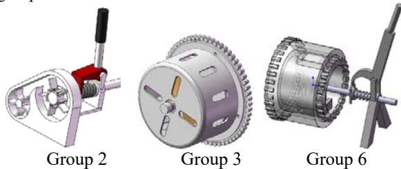
Figure 7. Clutch redesigned 3D modeling
