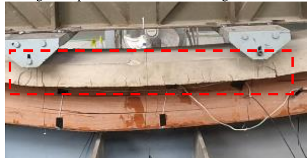
Figure 9 Failure mode of concrete slab
