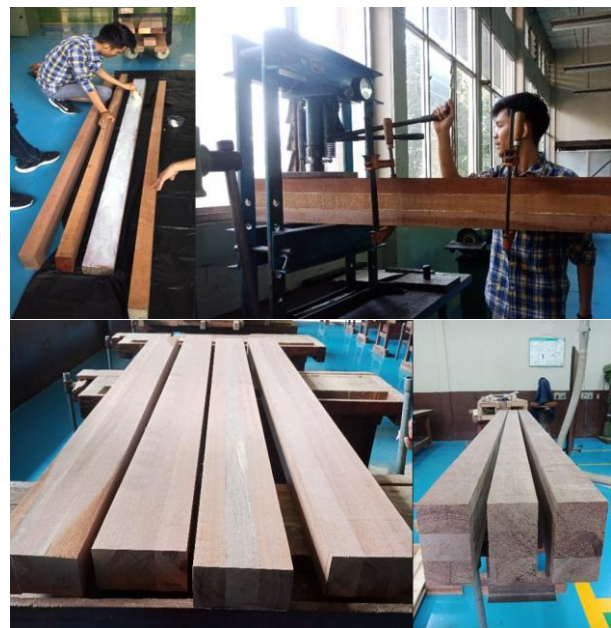
Figure 2 Glulam beam making process.
