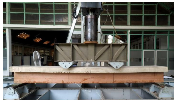
Figure 3 Setting up the composite beam test
