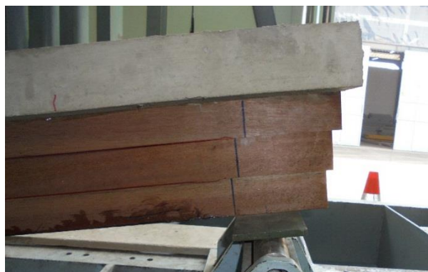
Figure 10 Damage along the adhesive plane of the glulam
