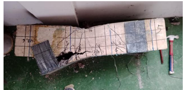
Figure 6 Seawater-immersed Concrete Failure Model
