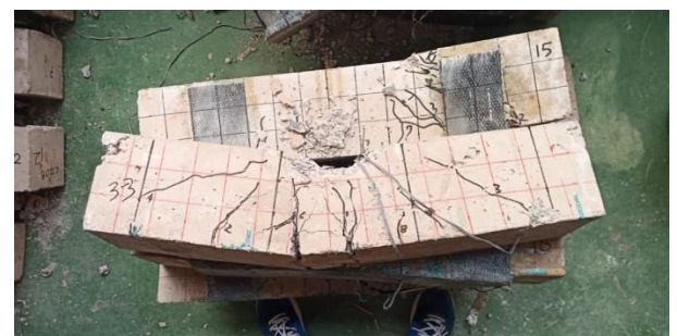
Figure 7 Normal Concrete Failure Model
