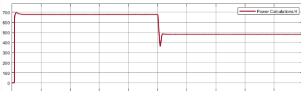
Figure 8 Load Power Stability (W)
