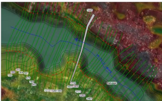
Figure 4. Geometric modeling (river and bridge)
