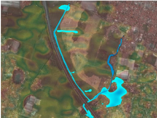
Figure 9. The return period of flood discharge is 2 years after having 2 box culverts
