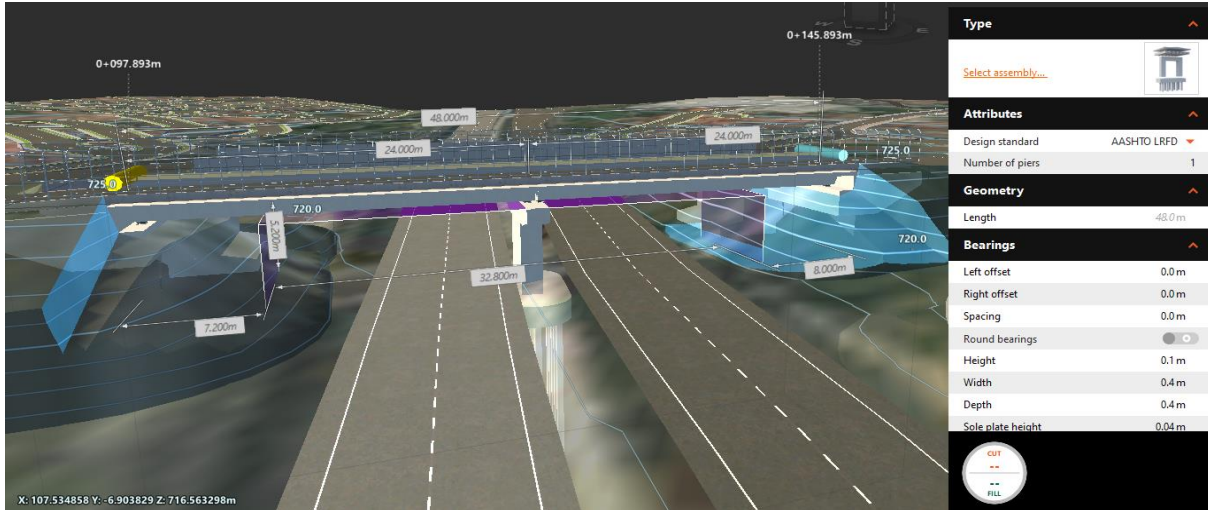
Figure 2 Existing Bridge Dimension Approach
