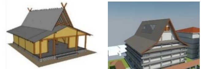
Fig. 4. The adoption of the rooftop shape for the development of the UPI Purwakarta Campus (Source: research data, 2020).
