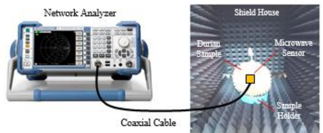
Fig. 12. Experimental setup of durian maturity measurement, where vector analyzer was used to be a generator to feed swept microwave band through coaxial cable into microwave sensor, and then to measure durian sample. The experiment was done in the shield house to avoid noises and interferences.
