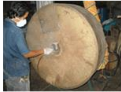
Fig. 1. Glue spraying in a glue mixer.
