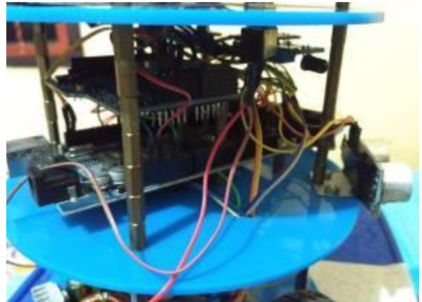
Figure 4. 2nd Level, Arduino, XBee, and Ultrasonic Sensor
