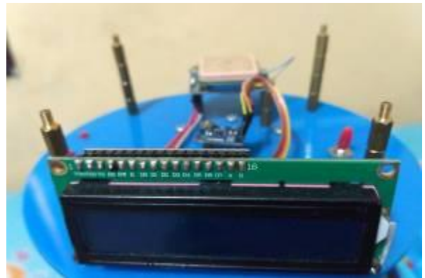
Figure 5. 3rd Level, LCD 16x2, Compass, and GPS
