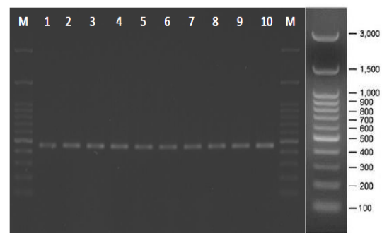
Figure 2 Electrophoretic profile for the MSTN gene fragments amplified by PCR in a 1% TBE agarose gel. (M:1kb DNA ladder; Lane 1-10 represented a strand with 463 bp).
