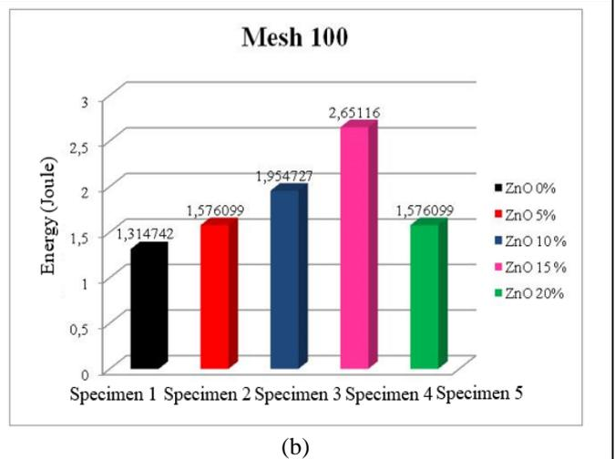
Fig. 2. Comparison of impact value with EFB meshing size 80 and 100.
