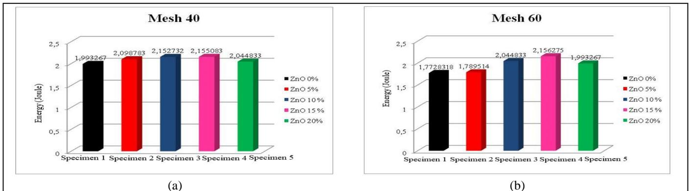
Fig. 1. Comparison of impact value with EFB meshing size 40 and 60.
