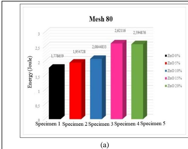
Figure 2(a) shows that the impact test of each specimen with 80 mesh of EFB absorbs Energy (E) more than 142.2928 Joules from the pendulum Charpy Work (w) on the pendulum to break the specimen worth 0.011383 kg.m. The diagram shows that specimen 4 with EFB 80 mesh size and 15% ZnO also shows the highest impact value of the five compositions of the test specimen is specimen 4 with a value of 2.62116 Joules.
