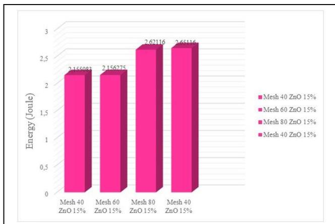
Fig. 3. Comparison of impact values based on EFB fiber size.
