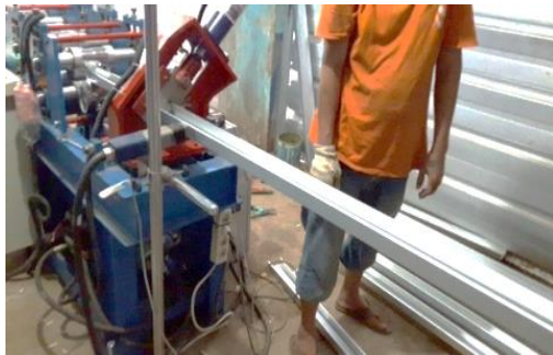
Fig. 3. The manufacturing process of lightweight structural steel profiles in Indonesia [9].
