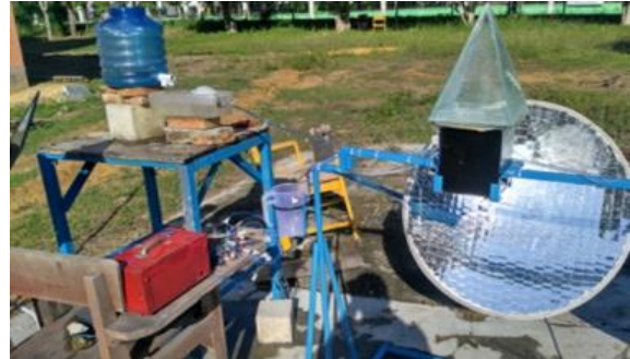
Fig. 1. Seawater desalination test device with a parabolic reflector.
