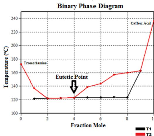
Figure 1. Eutectic point of caffeic acid-tromethamine mixture
